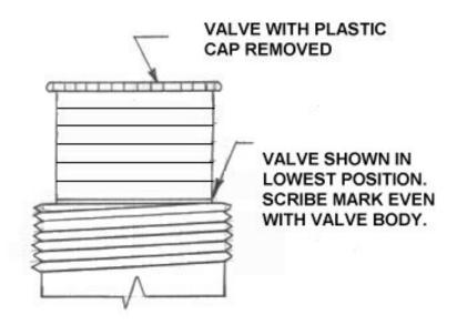
The valve may need to be cleared of dirt or chips if adjustment is not possible. With the compressor running, turn the valve adjustment knob clockwise about 3 turns momentarily then back to the proper setting. Do not leave the valve in the open position allowing high backpressure, as this may cause the compressor to overload.
